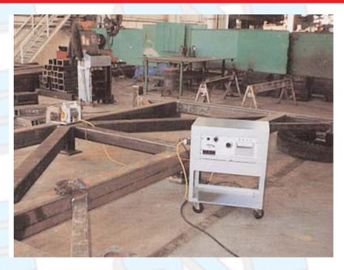
introduced into the material in one or more of the following ways: thermal, metallurgical, mechanical and chemical. Since these are the processes that make up our metalworking trades, it is only right to assume that, at some point in time, a stress relief treatment may be required.
